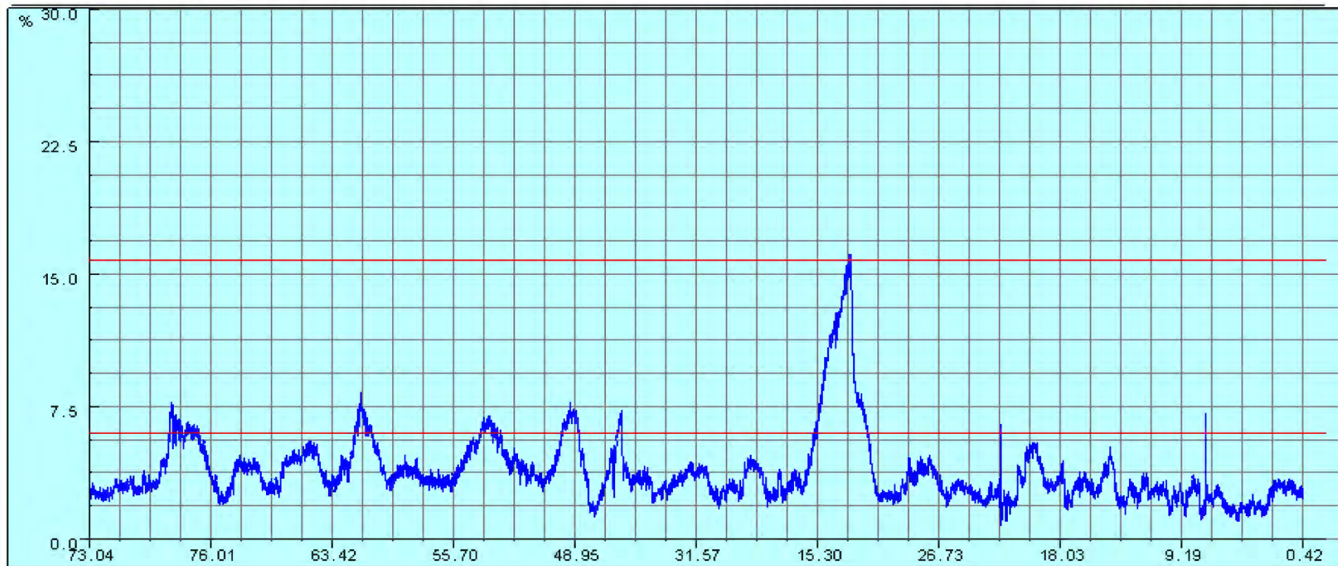
Ovality(q)* as a percentage of original pipe versus time (frame number) m
