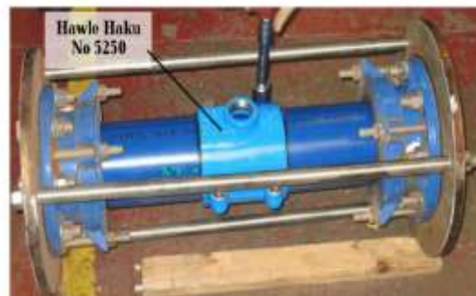
Figure 2, Test rig for Hawle Ferrule strap
