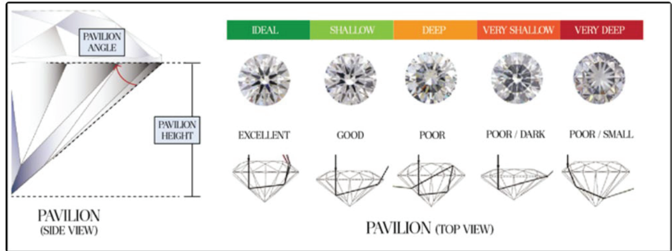
The pavilion of a diamond redirects light back to the observer and the wearer
