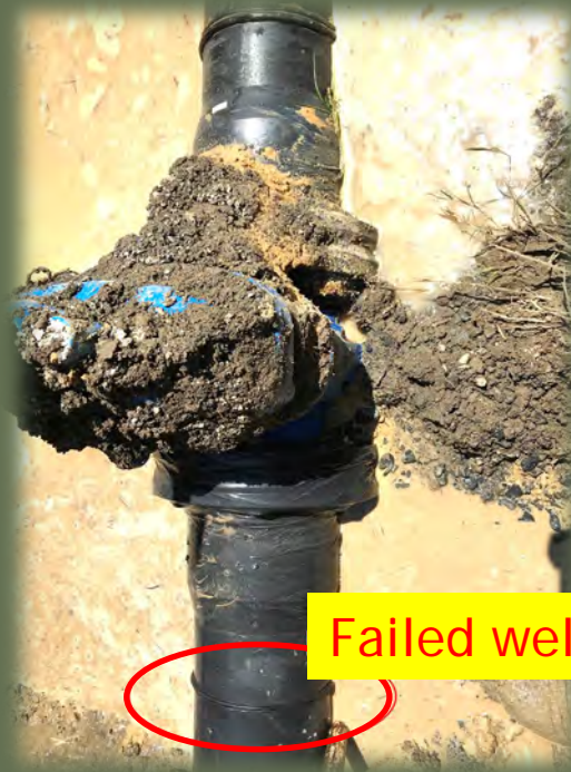
Not enough pressure during welding / cool time.
