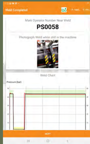
Photo of completed weld and review
