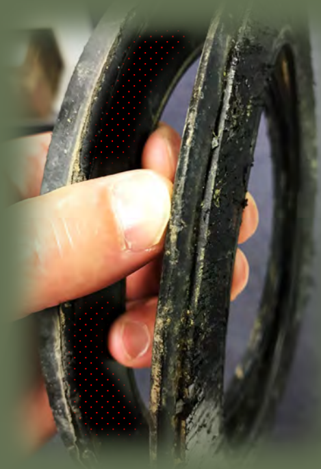
Too much pressure during heat soak phase
