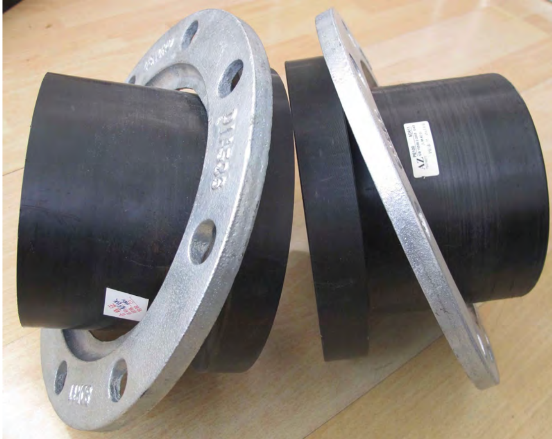
Typical pair of moulded HDPE stub flanges (for butt welding) and Ductile Iron Flanges (bolts and nuts not shown)
