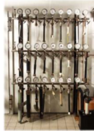
The first creep rupture tests on pipes made from HDPE were already started in 1955
