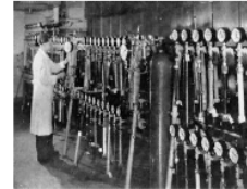
On October 18th 2012, two pipe specimens in this "historical" test have celebrated their 56th anniversary of continuous testing!
