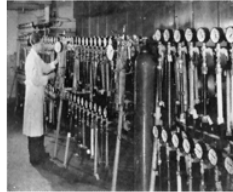
Creep Rupture tests on HDPE pipes started already in 1955
