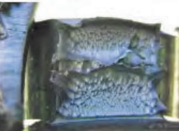
Figure 2: showing fully ductile failure mode of tensile weld specimen
