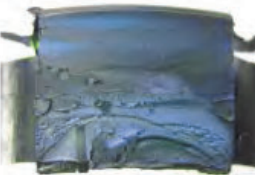
Figure 3: showing "mixed" and brittle failure modes of tensile specimen
